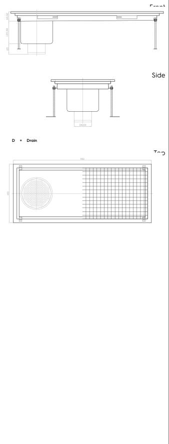
Floor Drains and Collecting Tanks Floor Drain with Stainless Steel Grate and Side Drain - Vertical outlet 400x950 mm The company reserves the right to make modifications to the products without prior notice. All information correct at time of printing.
